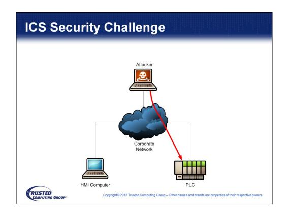
Imagine a manufacturing line, where a physical process is controlled by a digital component called a Programmable Logic Controller (PLC). The other piece of that system is an operator display panel, the Human Machine Interface (HMI), which is typically physically remote from the actual process that needs monitoring. As we see changes in the process, we should be able to see the operator display update in real-time.
