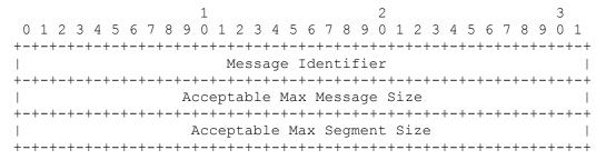
Figure 13 - Segmentation Contract Rejected Error Information
