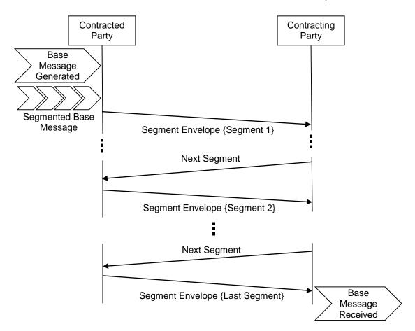
Figure 3 - Segmented Message Exchange
