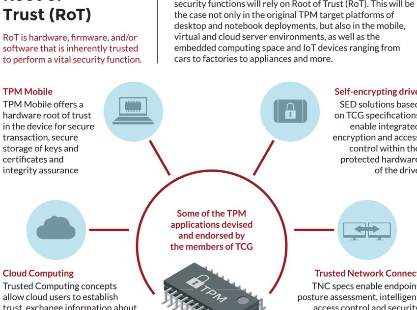
TPM Mobile: TPM Mobile offers a hardware root of trust in the device for secure transaction, secure storage of keys and certificates and integrity assurance.
