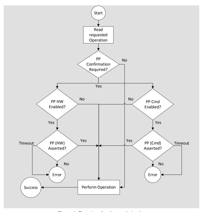
Figure 1: Flowchart for timeout behavior
