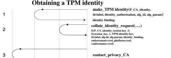
The TPM creates an identity-binding signature (the value of a signature over the TCPA\_IDENTITY\_CONTENTS structure). Among other things, this proves possession of the new private key, which does the signing of the TCPA\_IDENTITY\_CONTENTS structure. The Subsystem sends the signature along with evidence of a genuine TPM and the platform the TPM resides on to a Privacy CA. The encryption of the request is to provide privacy not security.
