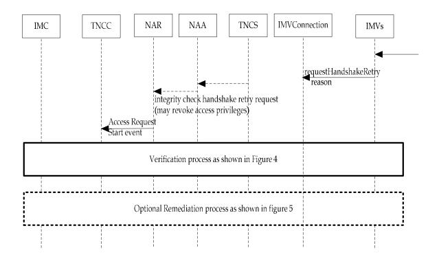
Figure 6 – Java Bindings: IF-IMV Handshake Retry Initiated by TNCS
